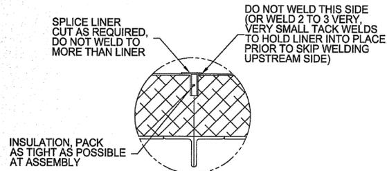
TYPICAL INNER LINER LAP AT FIELD JOINT DETAIL
